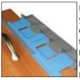
It's also worth considering replacing the handles. This will make your new doors look even better and add a lot of value to the completed job. When fitting the handles always remember to drill from the front to back. It may be a good idea to purchase a handle position drilling jig which will show you how to position the handles accurately on all your doors.
