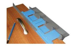
Set up the drilling jig to line up with the holes on the handles that you are planning to use. Hold the handle against the jig so you can see which holes to use. On the right, you can see that the first and fourth holes correspond with a 96mm hole centre of this particular handle. Then you need to drill out the first and the fourth hole on the jig using a 3mm drill bit.
