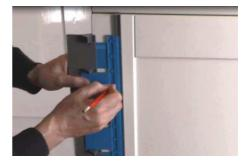
It takes a couple of minutes to set up the drilling jig, but once you've done it, it will help you mark all the other holes on all the doors without having to take any more measurements. To mark a door of the opposite hand, simply turn the jig around, and to mark a wall unit door simply flip the jig over.
