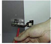
The front screw on the hinge is normally used to adjust door alignment, or in other words, the distance that the door overlays the cabinet. Its this adjustment that moves brings the door closer too, or further away from the edge of the cabinet.
