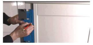
It does take a couple of minutes to set up the Handle Hole Drilling Jig but once it is set up its going to allow you to mark all the other holes on all the doors without having to take any more measurements. To mark a door of the opposite hand, simply turn the jig around. to mark a wall unit door simply flip it over.
