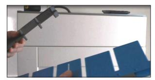
As an example, if the height of a drawer front is 140mm and the jig only expands to 65mm it's not going to expand to the 70mm (half of 140mm) that we want for marking the centre line.
