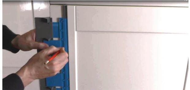
It does take a couple of minutes to set up the Handle Hole Drilling Jig but once it is set up its going to allow you to mark all the other holes on all the doors without having to take any more measurements. To mark a door of the opposite hand, simply turn the jig around. to mark a wall unit door simply flip it over.
